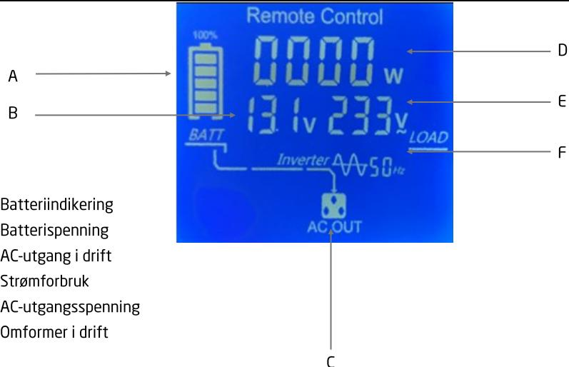
FJERNKONTROLDISPLAY OVERFØRINGSBRYTERMODUS (1000W / 1500W /2000W /3000W)
