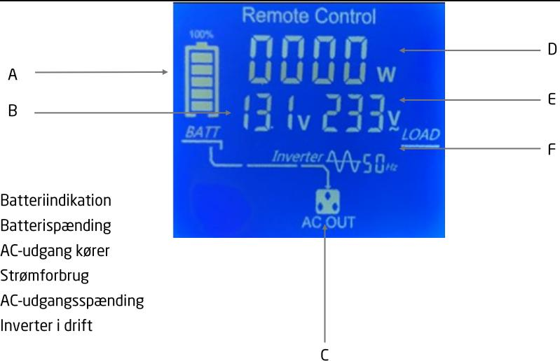
FJERNBETJENING DISPLAY TRANSFERSWITCH MODE (1000W / 1500W /2000W /3000W)
