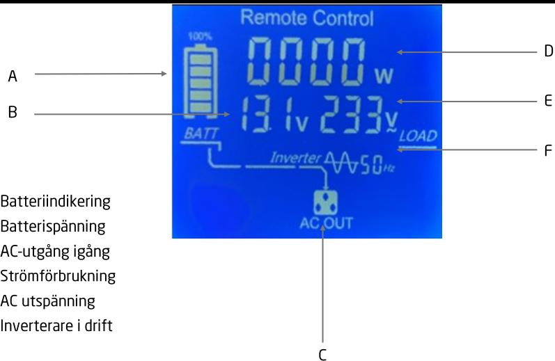
FJÄRRKONTROLL DISPLAY ÖVERFÖRINGSLÄGE (1000W / 1500W / 2000W / 3000W)
