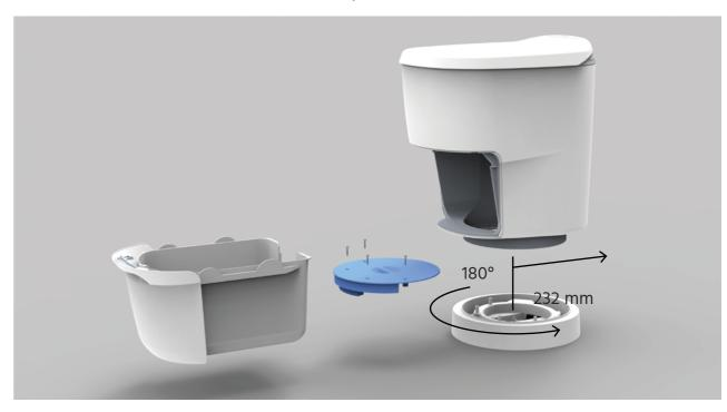
To allow for the opening of the lid in any rotational position, a minimum distance towards side walls and other installations must be kept. When using the round socket leave 232 mm between the rotational axis and the back wall. When installing the L-adapter leave 225 mm from the toilet's centre to any spatial limitations left or right.
